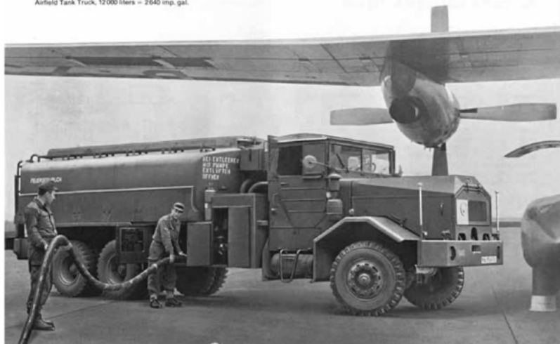
FAUN L908/ATW Airfield Tank Truck, 12000 liters = 2640 imp. gal.
