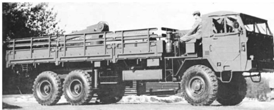
FAUN L908/ATW Airfield Tank Truck, 12000 liters = 2640 imp. gal.
